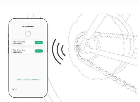
To turn The All In One on lift and turn the pedals or start pedaling.
