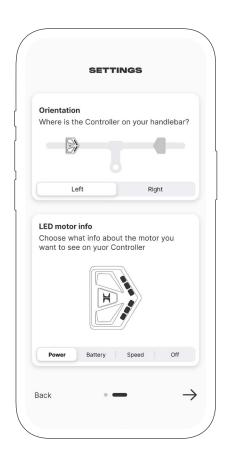
During the configuration you can set up the position of the remote controller on the handlebar and what to display on the six leds. These settings can be changed every time desired from the Controller page on the app.
